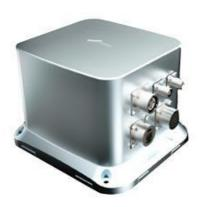
ER-7660 FOG INS built-in total temperature 0.3 °/ h high-precision closed-loop fiber optic gyroscope, 100 ug high precision quartz accelerometer. It supports BD function mobile mapping level multi-mode multi-frequency GNSS receiver, which can realize dynamic rapid alignment or GNSS double antenna auxiliary fast high precision orientation, which can be up to 0.1°.
